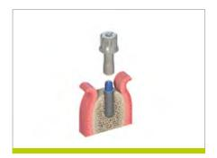
To extract the implant after the pre-determined breaking point broke, simply take out the broken part of the  $Loxim^{TM}$  from the adapter and re-insert the adapter on the  $Loxim^{TM}$  part remaining in the implant. Counterclockwise turns will remove the implant.
